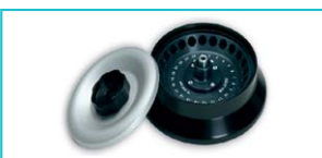
Item: Z216-2420H 24 x 1.5/2.0ml Angle Rotor (45°) Hermetically Sealed Lid Max Speed: 15,000 rpm / 21,379 x g Accel: 21 sec. / Decel: 21 sec.
