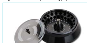
Item: Z216-4420 44 x 1.5/2.0ml Angle Rotor (32°/55°) Max Speed: 15,000 rpm / 21,379 x g Accel: 25 sec. / Decel: 17 sec.
