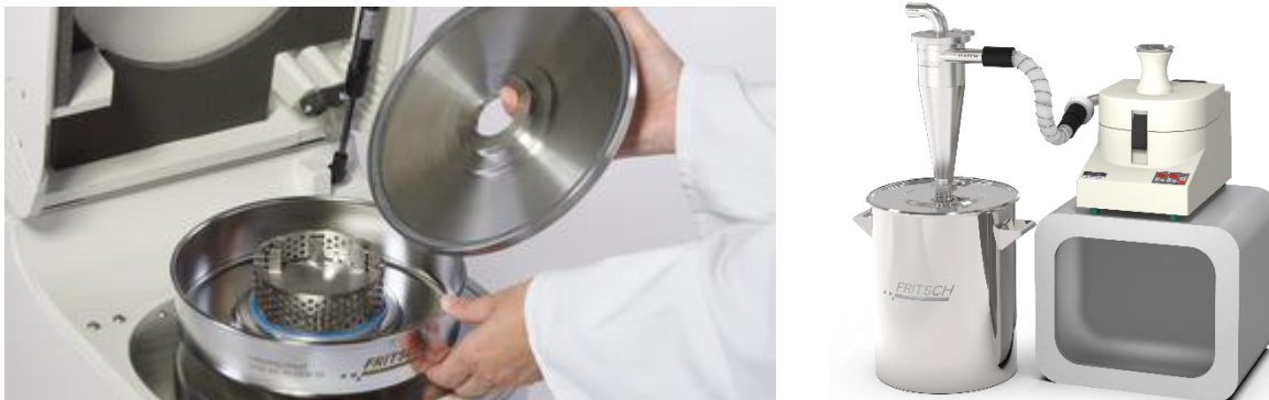
Fig. 1: Inside of PULVERISETTE 14 rotor mill, showing fixed collection pan, rotor, and sieve ring. High performance Cyclone sample collector in stainless steel is shown on the right. Used together with modified collection pan, the P14 system & Cyclone allow continuous feeding & homogenization of CBD material into the low micron range (consistency of talcum powder).
