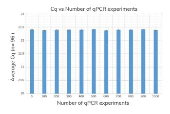
Robust design. After sequential sets of 1000 continuous qPCR experiments, a GAPDH qPCR assay was performed and Cq values were recorded at every 100 experiments points. Average Cq in each assay = 22.4, ±0.01.
