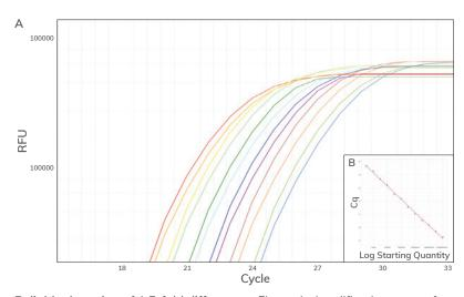
Reliable detection of 1.5-fold differences. Figure A. Amplification curves for assays of GAPDH in a dilution series of human reference cDNA (n=3). Assays were conducted using BioRad<sup>TM</sup> Sso Advanced SYBR Green Mix®. Figure B shows the standard curve obtained by plotting Cq values vs the amount of template DNA (copies/ $\mu$ I). R²=0.998, efficiency = 99.89%.
