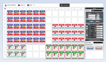
Quickly set up and confirm plate layout. Each well is color coded by sample type, biological replicate, and technical replicate. Well type and standard curve values are also easily visible.
