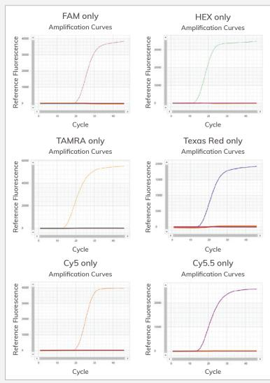
Multiplex qPCR reaction were scanned for all 6 channels in an Azure Cielo Real-Time PCR system. Single channel amplification curves were as expected, with no signal leakage or crosstalk.
