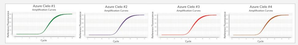
Reproducible data on four separate Azure Cielo instruments using Human GAPDH assay and SYBR Green Master Mix. Average Cq = 20.11, SD= 0.002
