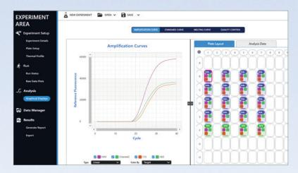
View each individual amplification trace by target or sample. Easily adjust threshold values by dragging the threshold line, or typing in the threshold value.
