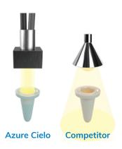
Single illumination light sources can deliver light both in and out of the wells, resulting in higher background, and less light hitting the sample. Azure Cielo uses fiber optics to directly deliver light to each indivdual well.
